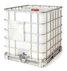
An Intermediate bulk container (IBC) is a container used for transport and storage of fluids and bulk materials. IBC's range in size but are generally between 700 and 2,000 mm (27.6 and 78.7 in) or 46 to 52 in (1,168 to 1,321 mm) in height. The length and width of an IBC is usually dependent on the pallet dimension standard of a given country.
